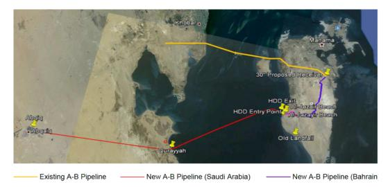
The front-end engineering design of the pipeline was completed in 2014 and separate contracts were awarded for the 43-kilometre long onshore Saudi Arabia stretch of the pipeline, the 41-kilometre offshore stretch and the 28-kilometre onshore Bahrain stretch. The new pipeline was completed and commissioned in October 2018, at which point decommissioning of the existing older pipeline commenced.
